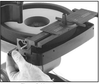
Figure 5. Mounting tool rest.
